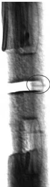
Figure 11.30 Three-dimensional image of specimen B (3-mm crack), showing the crack extension through the whole thickness of the sample.
